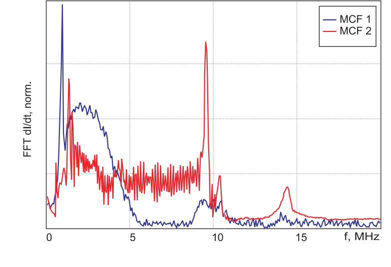
Experiment MCF #1 demonstrates that operation of helical FCG with a capacitive load corresponds in general analysis [1], but additional losses [2] present in the circuit drastically reducing initial current and radiation frequency.
