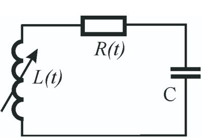
Operation of FCG with a capacituve load (magneto-cumulative generator of frequency (MCF)) is accompanied by radiative and diffusive losses. With the growth of operation frequency of MCF, the influence of losses increase and form <a href="fish"-like dependence">fish"-like dependence of the amplitude of current on operation time.</a>
