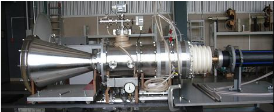
Experimental prototype of virtual cathode oscillator provides 200 MW peak output power in frequency range from 2.5 to 5 GHz
